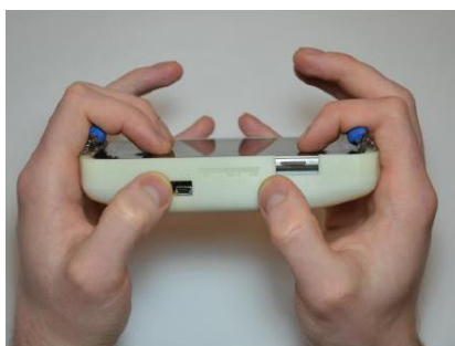
Figure 8 - The system consists of six vibrotactile motors attached to springs and a 3D-printed case. The springs mould to users' hands and dampen vibrations through the device allowing better stimuli discrimination. (Nicolau et al. 2015)
