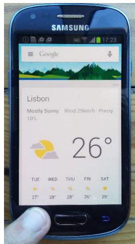
Figure 16 - Samsung S3 mini with two capacitive buttons with no feedback
